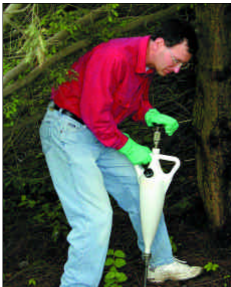
Kioritz Low Volume Soil Injection System
