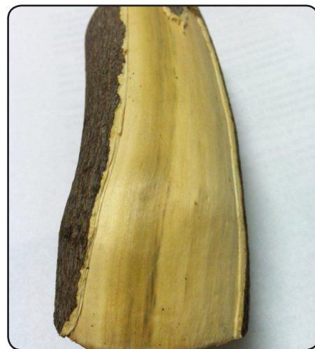
Staining is visible under bark
