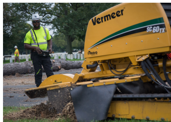
Stump grinder controlled by remote.
