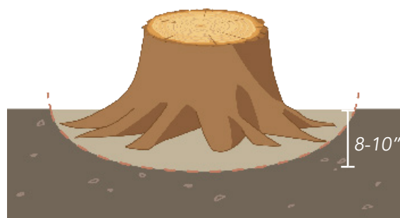
Grinding the stump down to 8-10" below the soil surface
